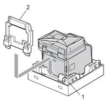
Place the upper carton (1) over the machine and the lower carton (2). Align the joint holes of the upper carton with the joint holes of the lower carton. Secure the upper carton to the lower carton using the four plastic joints (3) as shown in the illustration.
